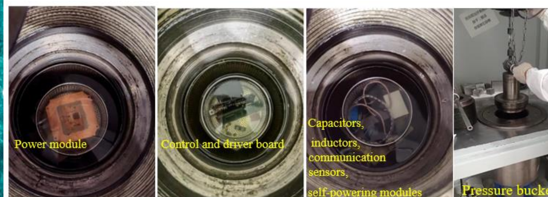
Pressure bucket with automatic increase and decrease of water pressure Water pressure test(30MPa, 60MPa)
