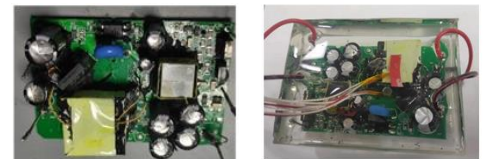
Improved self-powering is directly potted with epoxy resin
